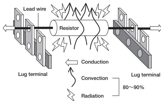
Figure 2. Heat dissipation of cylindrical resistors
