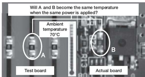
Figure 5. Temperature differs depending on the board
