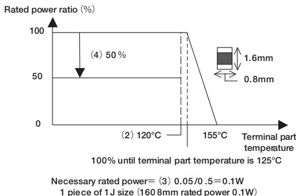
Figure 7. Selection using a terminal-temperature derating curve
