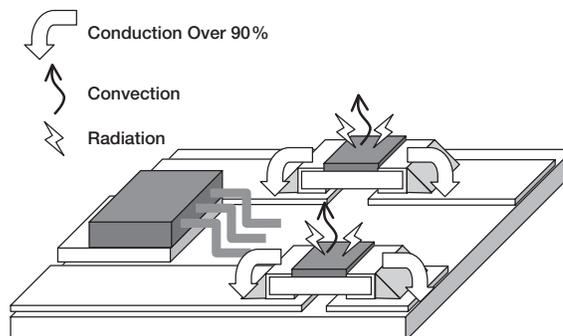
Figure 3. Heat dissipation of surface mount resistors
